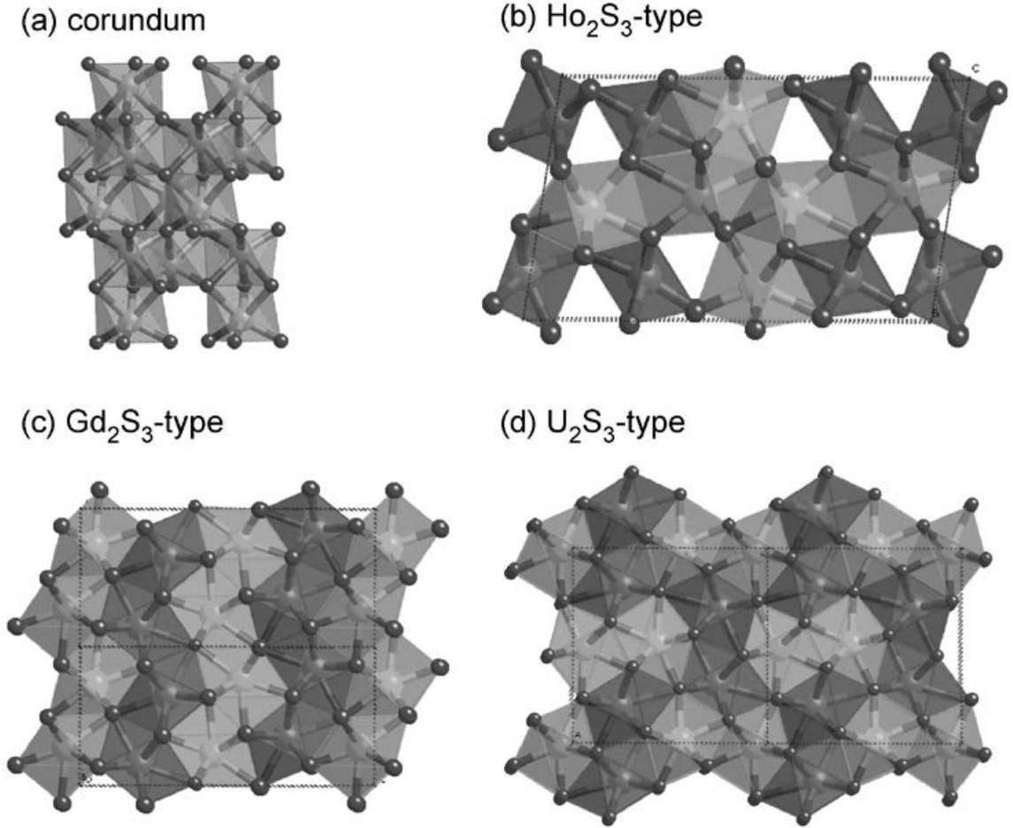
**Figure 12.** Crystal structures of  $R_2S_3$  (R: lanthanoid or actinoid). The coordination numbers of cations are 6 in corundum, 6 and 7 in Ho<sub>2</sub>S<sub>3</sub>-type, 7 and 8(=7+1) in Gd<sub>2</sub>S<sub>3</sub>-type and U<sub>2</sub>S<sub>3</sub>-type structures.
