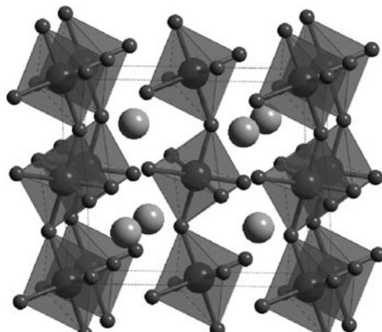
**Figure 1.** Structure of MgSiO<sub>3</sub> post-perovskite (PPV).
