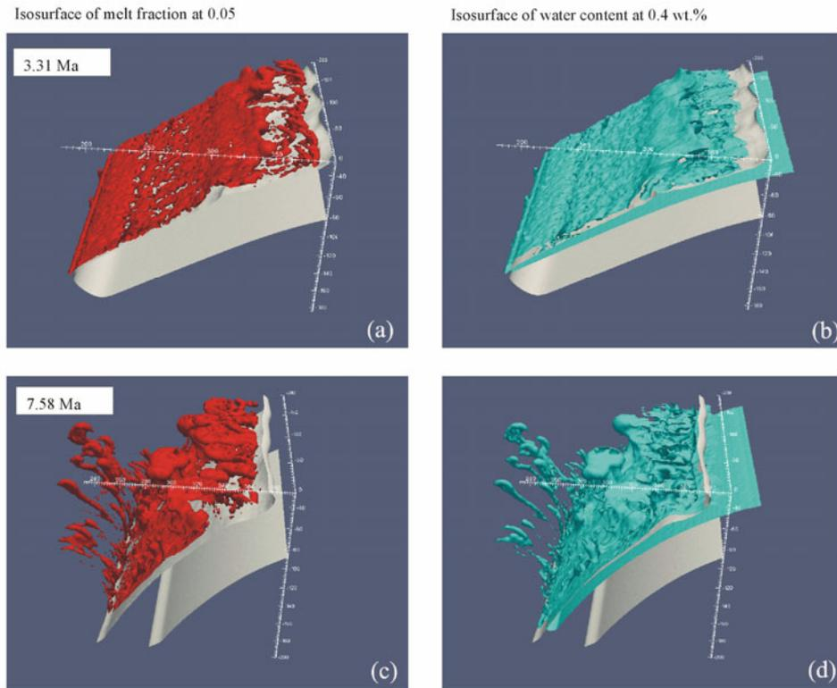
**Figure 3.** Evolution of melt and water content atop the subducting slab. Isosurface (in red) of melt fraction at 0.05 at 3.31 Ma (a) and 7.58 Ma (c). Isosurface (in blue) of water content at 0.4 wt.% at 3.31 Ma (b) and 7.58 Ma (d). The slab is defined by temperature isosurface at 750 °C shown in white gray.
