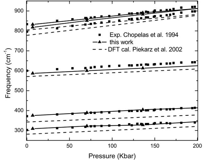
**Figure 3.** Pressure dependence of the Raman frequencies.
